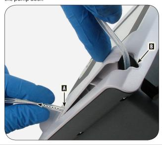
**15.** Attach the small end of the irrigation tube ⚠ to the handpiece irrigation fitting, following the instructions that came with your handpiece. Attach the irrigation tube to the motor cable at evenly spaced intervals using the AHP-03 clips ☑ provided in the AE-24 tubing set bag.
