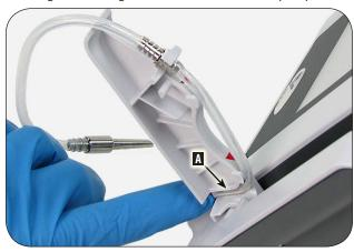
**14.** With one hand, pull the irrigation tube tightly from the bottom of the pump door **A**. Use the other hand to guide the irrigation tube into the notch **B** on the console while closing the pump door.
