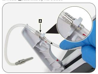
**13.** Following the next arrow on the door, thread the peristaltic tube segment through the bottom slot **A** on the pump door.
